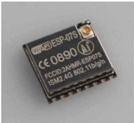
Figure 3 Top View of ESP-07s WiFi Module
