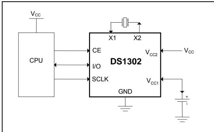
Figure 1. Block Diagram
